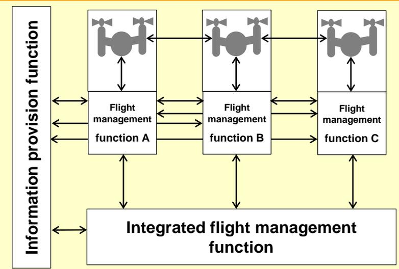
Conceptual image of drone flight control system
