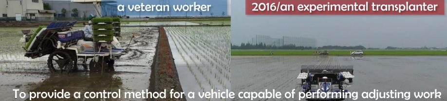
for the straight traveling and turning characteristics of the vehicle certainly and quickly with accuracy equivalent to a veteran worker.
